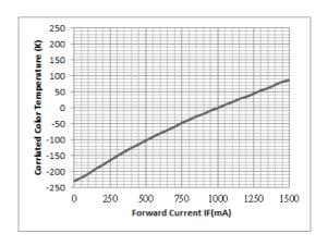
Fig 6. Correlated Color Temperature (CCT)Shift
