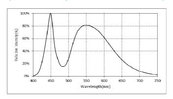
Fig 1. Relative Spectrum of Emission
