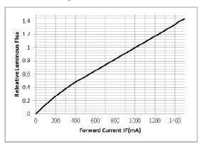
Fig 5. Relative Luminous Flux
