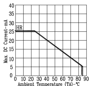
Fig5. MAX. ALLOWABLE DC CURRENT VS. AMBIENT TEMPERATURE.
