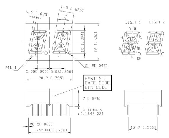
NOTES: 1. All dimensions are in millimeters. Tolerances are  $\pm\,0.25$  mm unless otherwise note.
