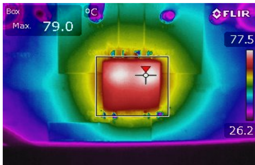
Figure 10. Thermal Image 12V to 1.0V, 36A with 200LFM without Heat Sink
