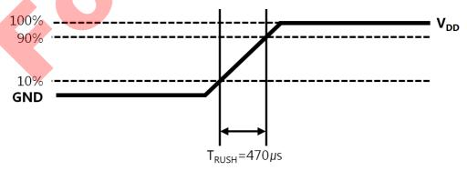
The rush current,  $I_{RUSH}$  can be measured when  $T_{RUSH}$  is 470  $\mu$ s.
