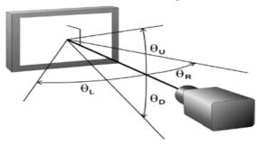
Note (6) Definition of Viewing Angle : Viewing angle range (C/R ≥ 10)
