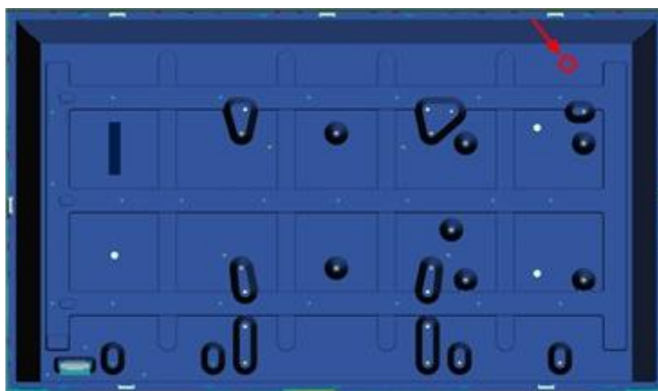
<Module Depth Measure Point>
