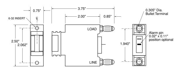
Dimensions for reference only. For additional options and dimensions, contact the factory.
