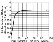
0 1 20 40 60 80 100 Peak Current(IP)-mA (AVG ≤10mA) Fig2. RELATIVE LUMINOUS EFFICIENCY (LUMINOUS INTENSITY PER UNIT CURRENT) VS. PEAK CURRENT
