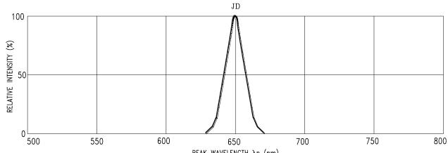
PEAK WAVELENGTH λp (nm) Fig1.Spectral Emission
