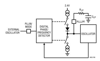
Figure 8. Phase-Locked Loop Block Diagram
