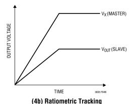
Figure 4. Two Different Modes of Output Voltage Tracking
