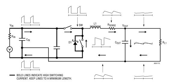
Figure 10. Branch Current Waveforms
