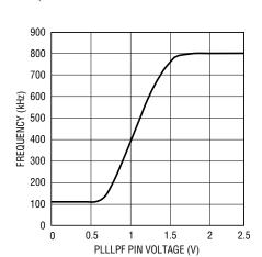
Figure 7. Relationship Between Oscillator Frequency and Voltage at the PLLLPF Pin When Synchronizing to an External Clock
