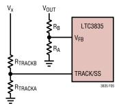
Figure 5. Using the TRACK/SS Pin for Tracking
