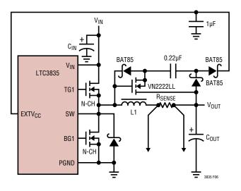
Figure 6. Capacitive Charge Pump for EXTV<sub>CC</sub>
