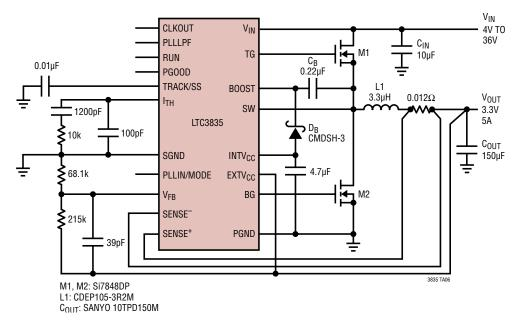
Figure 11. High Efficiency Step-Down Converter
