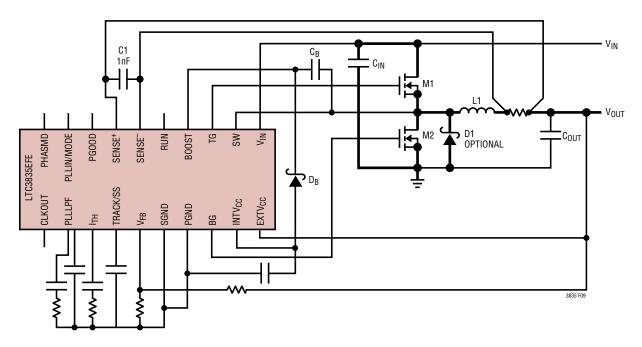
Figure 9. LTC3835 Recommended Printed Circuit Layout Diagram
