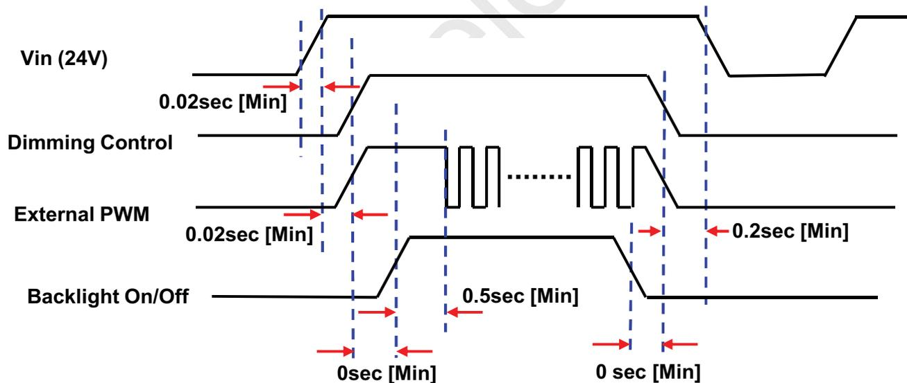
Note) SEQUENCE : ON = Vin(24V) > Dimming Control ≥ Backlight On/Off
