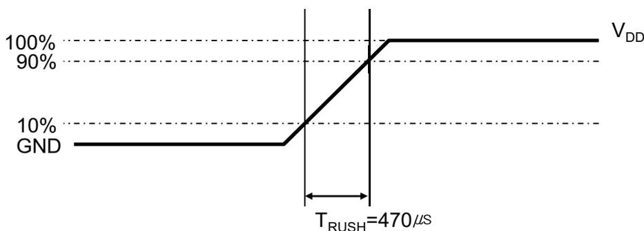
Rush Current  $I_{RUSH}$  can be measured when  $T_{RUSH}$  is  $470\mu\text{s}$ .
