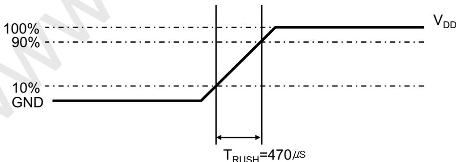
Rush Current  $I_{RUSH}$  can be measured when  $T_{RUSH}$  is  $470\mu\text{s}$ .
