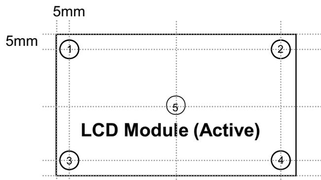
$\Delta T$  should be less than  $10\text{ }^{\circ}\text{C}$  ( $\Delta T = |T_{\text{OPR}} - T_{\text{MAX}}|$ )
