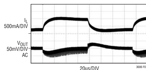
Figure 7. Transient Load Response of the LT3686 with Different Output Capacitors as the Load Current Is Stepped from 0.25A to 1A. V_{IN} = 12V , V_{OUT} = 3.3V , L = 6.8\mu H , Frequency = 2MHz
