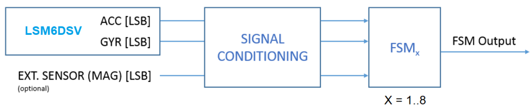
Figure 3. State machine in the LSM6DSV
