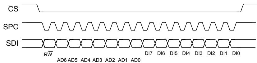
The SPI write command is performed with 16 clock pulses. A multiple byte write command is performed by adding blocks of 8 clock pulses to the previous one.
