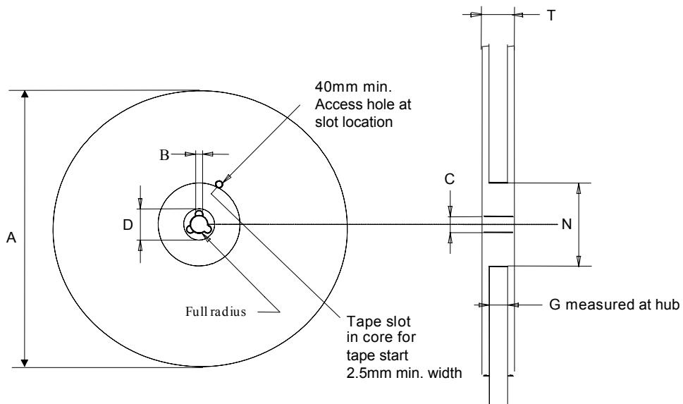
Table 471. Reel dimensions for carrier tape of LGA-14 package
