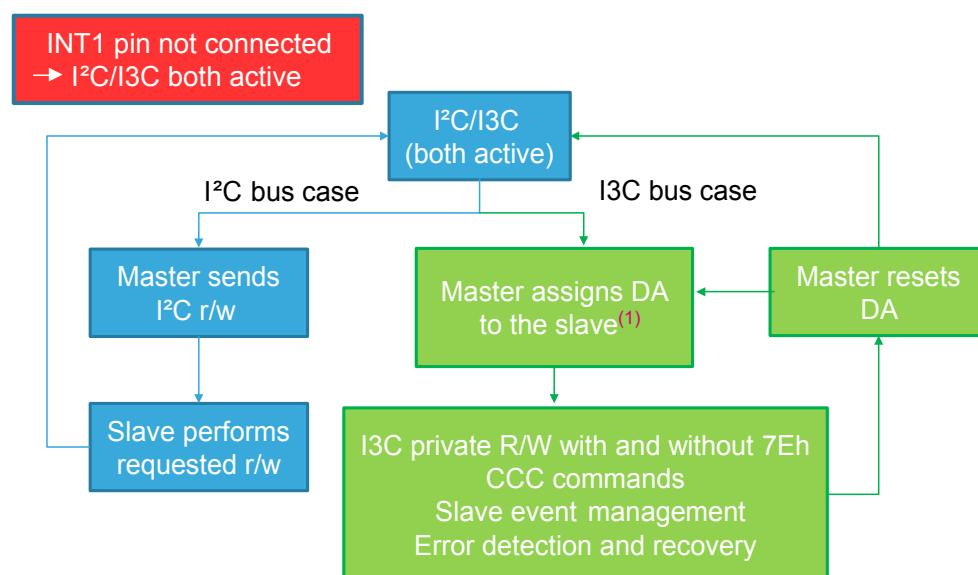
1. Address assignment (DAA or ENTDA) must be performed with I<sup>2</sup>C fast mode plus timing. When the slave is addressed, the I<sup>2</sup>C slave is disabled and the timing is compatible with I3C specifications
