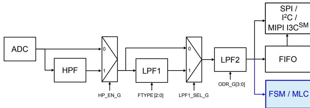
In this configuration, the gyroscope ODR is selectable from 12.5 Hz up to 6.66 kHz. A low-pass filter (LPF1) is available if the auxiliary SPI is disabled, for more details about the filter characteristics see [Table 61. Gyroscope LPF1 bandwidth selection](#).
