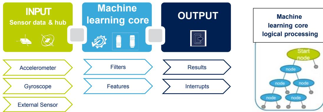
The LSM6DSTX can be configured to run up to 8 flows simultaneously and independently and every flow can generate up to 16 results. The total number of nodes can be up to 256.
