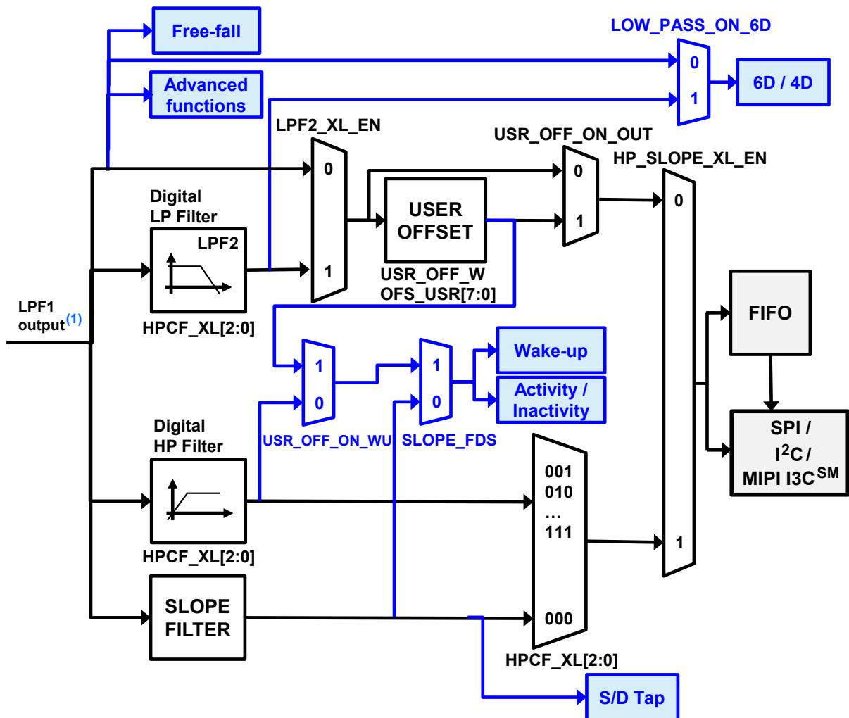
1. The cutoff value of the LPF1 output is ODR/2 when the accelerometer is in high-performance mode. This value is equal to 700 Hz when the accelerometer is in low-power or normal mode.
