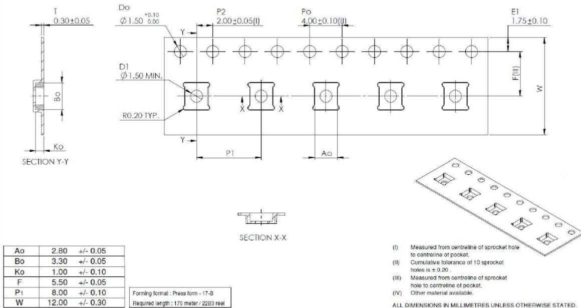
Figure 30. LGA-14 package orientation in carrier tape
