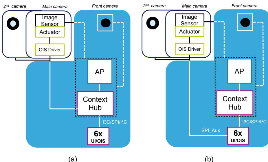
Then, the AP can configure OIS functionalities through `UI_INT_OIS` (6Fh), `UI_CTRL1_OIS` (70h), `UI_CTRL2_OIS` (71h), `UI_CTRL3_OIS` (72h).
