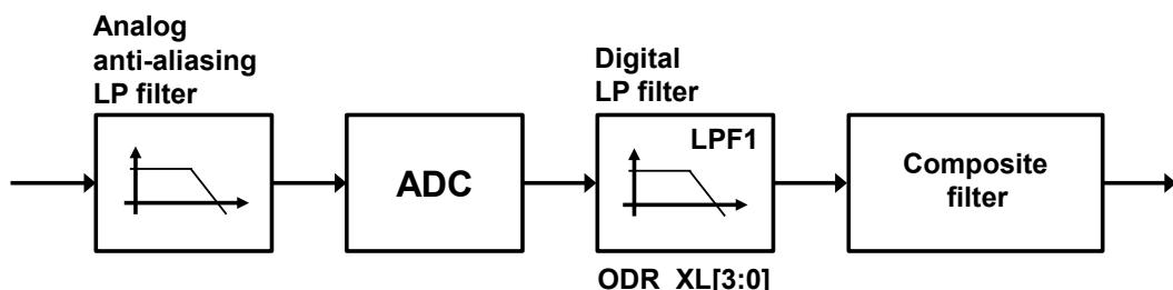
Figure 18. Accelerometer composite filter
