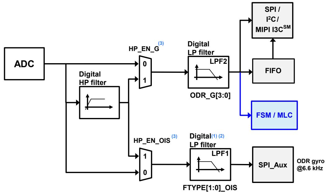
1. When mode3/4 is enabled, the LPF1 filter is not available in the gyroscope UI chain.
