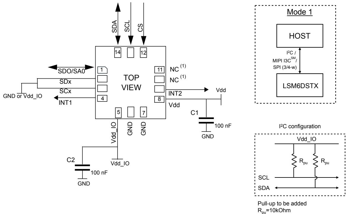
1. Leave pin electrically unconnected and soldered to PCB.
