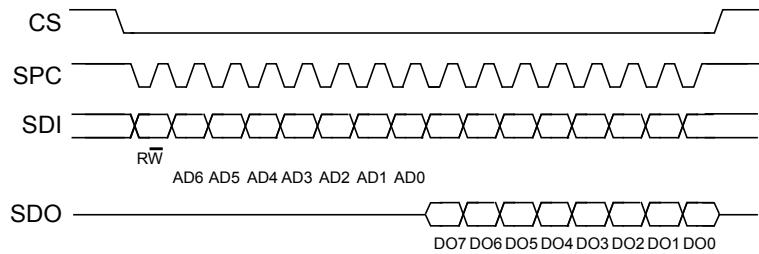
The SPI read command is performed with 16 clock pulses. A multiple byte read command is performed by adding blocks of 8 clock pulses to the previous one.
