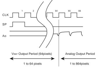
Note) Output blank part cannot be used as the analog output standard level.
