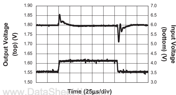
Step-Down Converter Line Transient ( V_{OUT} = 1.8V @ 400mA; EN = V_{IN} ; ENLDO = GND )
