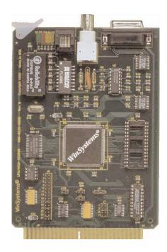
with the IEEE 802.3 standards. Supported interfaces include both the Thin and Thick Ethernet and Twistedpair Ethernet (10BASE-T) on a single STD Bus board.
