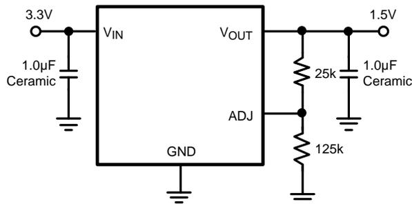
Figure 2. Adjustable  $V_{OUT}$
