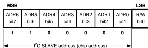
Figure 41. I 2 C Chip Address (see note above)
