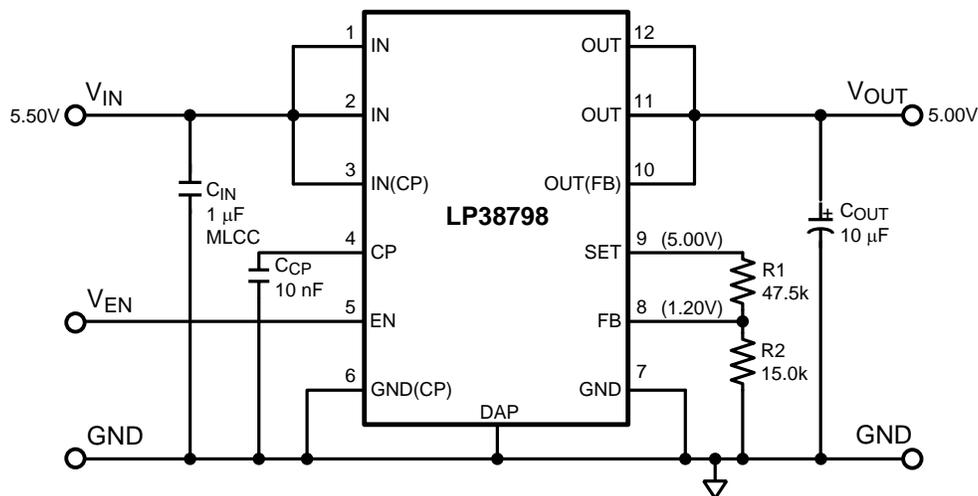
Figure 40. Typical Application,  $V_{OUT} = 5\text{ V}$
