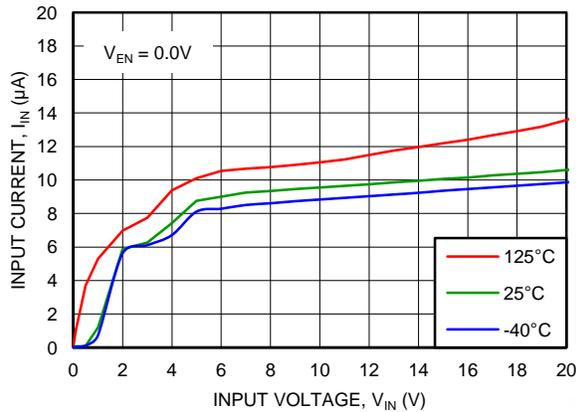
Figure 19. IN Pin Current vs  $V_{IN}$
