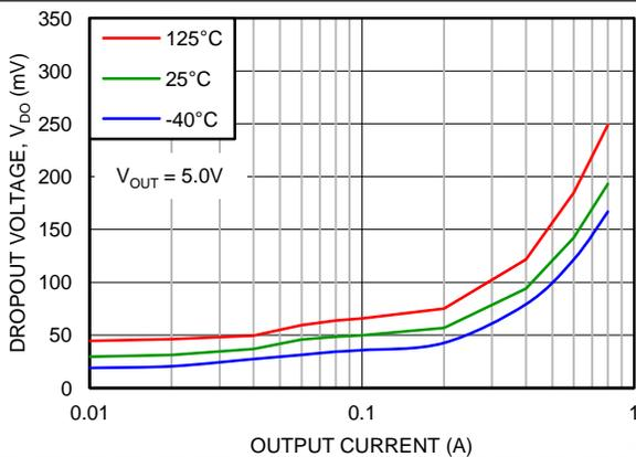
Figure 23. Dropout Voltage vs Output Current
