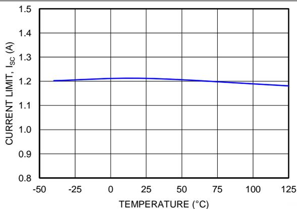
Figure 27. Current Limit,  $I_{SC}$  vs  $T_J$
