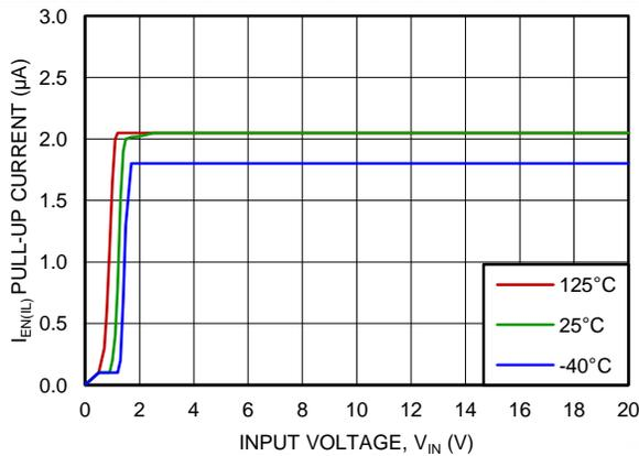
Figure 21. Enable Pin Pull-Up Current vs  $V_{IN}$
