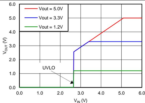
Figure 17.  $V_{OUT}$  vs Rising  $V_{IN}$
