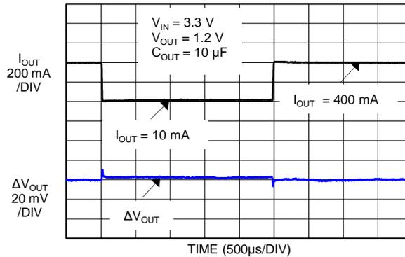
Figure 39. Load Transient
