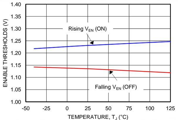
Figure 12. Enable Thresholds vs  $T_J$
