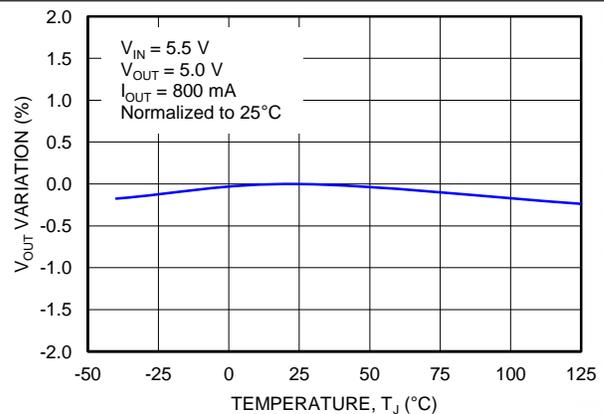
Figure 24.  $V_{OUT}$  Variation vs  $T_J$
