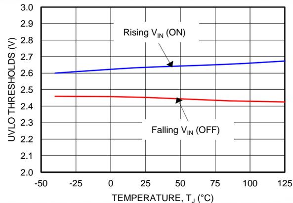
Figure 11. UVLO Thresholds vs  $T_J$
