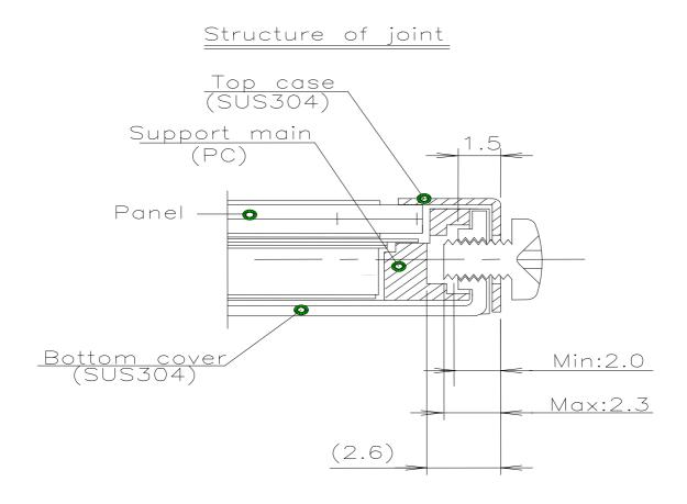
\* Mounting Screw depth : 2.0[mm] Min. 2.3[mm] Max.
