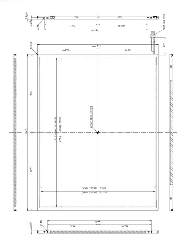
Notes 1. Unspecified dimensional tolerance are  $\pm 0.5 \text{mm}$
