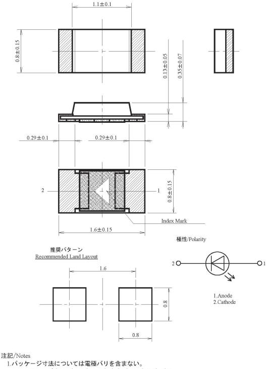
Measurement of the package doesn't include electrode projection.
