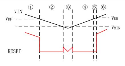
Delay time can be set by external capacitor Tdly= $3.8 \times 10^{-6} x C_{SR.}$
