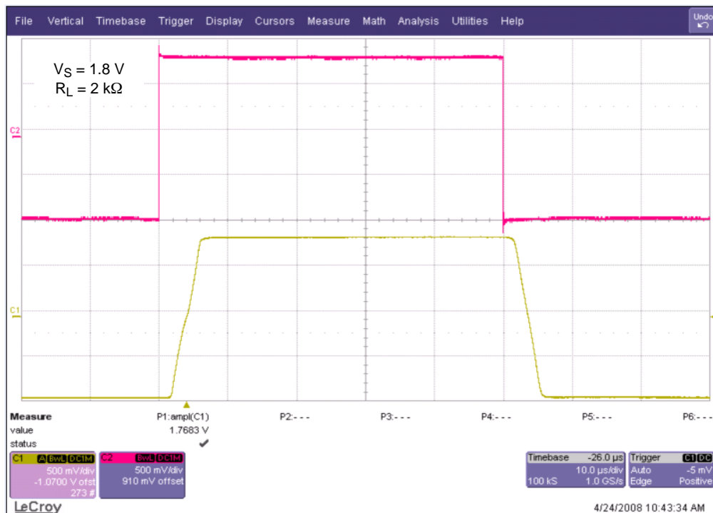
Figure 18. Small Signal Noninverting Response
