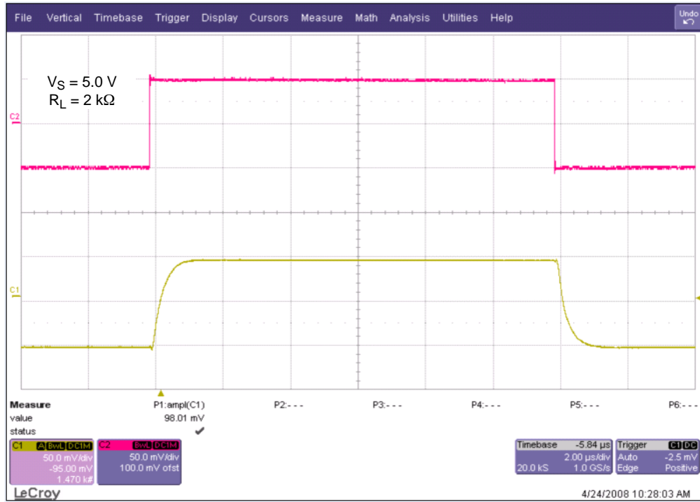
Figure 18. Small Signal Noninverting Response
