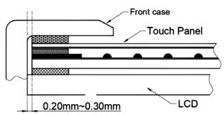
In general design, touch panel V.A. should be bigger than the LCD V.A. and touch panel A.A. should be bigger than the LCD A.A.
