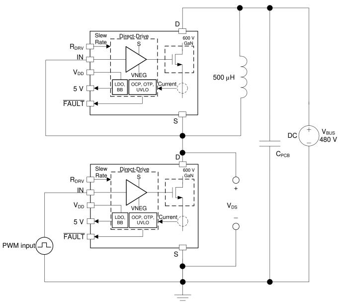
Figure 11. Circuit Used to Determine Switching Parameters
