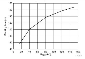
Figure 10. RDRV vs Blanking Time
