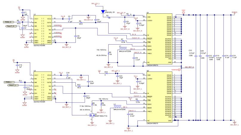
Figure 14. Typical Half-Bridge Application
