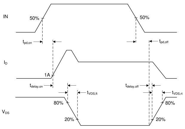
Figure 12. Measurement to Determine Propagation Delays and Slew Rates
