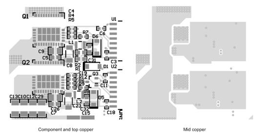
Figure 19. Example Half-Bridge Layout
