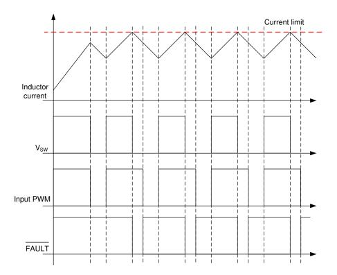
Figure 13. Cycle-by-cycle OCP Operation
