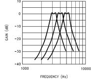
FIGURE 1. Response curves for the three filters in the LMF380. The clock frequency is 250 kHz.
