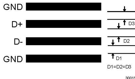
FIGURE 9. Ideal Diode Trace Layout
