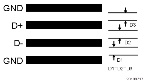
FIGURE 4. Ideal Diode Trace Layout
