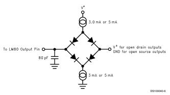
FIGURE 3. Digital Output Load Test Circuitry
