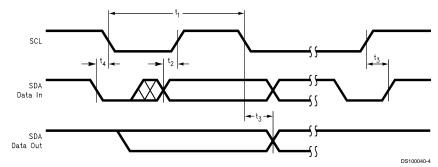
FIGURE 1. Serial Bus Timing Diagram
