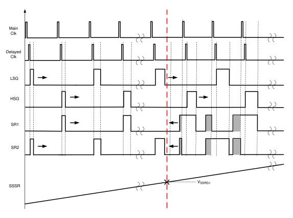
Figure 7-10. PWM Timing During Startup Process
