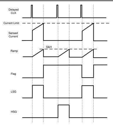
Figure 7-14. Pulse Matching Operation
