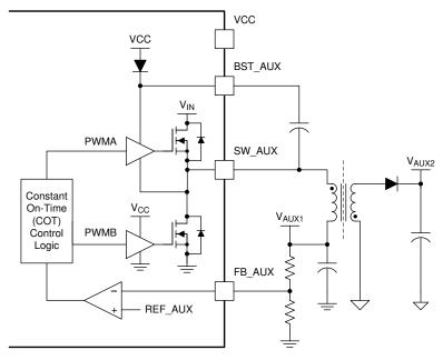
Figure 7-22. COT Controlled Fly-Buck Auxiliary Supply Circuitry
