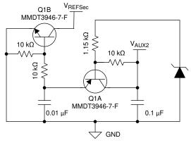
Figure 8-3. Secondary Auxiliary Voltage Level-Shift Detection Circuit
