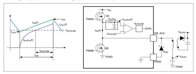
Figure 7-25. Aux Current Limit Circuit Model
