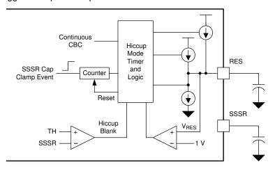
Figure 7-17. Hiccup Mode Circuitry
