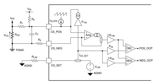
Figure 8-7. Current Limiting Block
