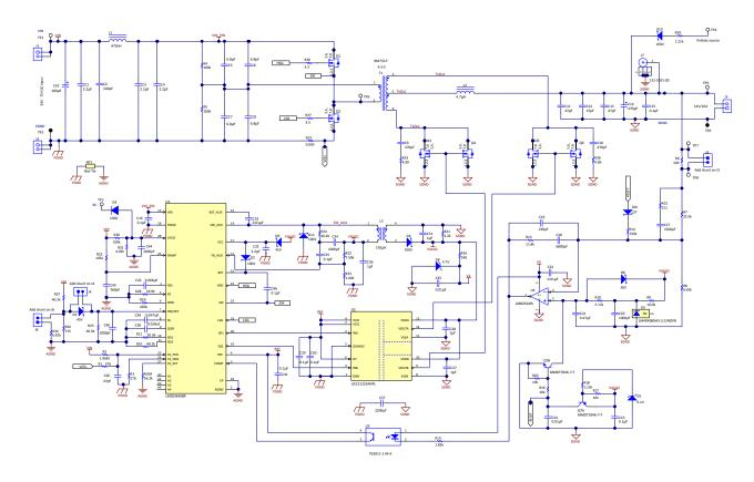
Figure 8-1. Evaluation Board Schematic
