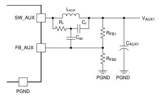
Figure 7-27. Minimum Ripple Configuration
