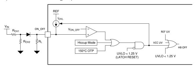
Figure 7-20. ON/OFF Pin Latch Function
