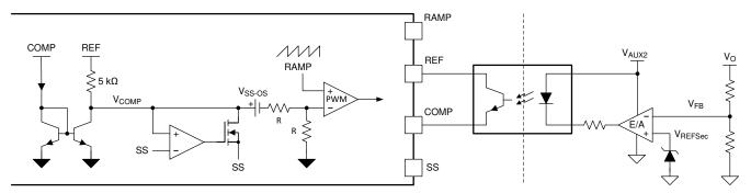
Figure 7-2. Voltage-Mode Feedback Control Loop for Half-Bridge Converter
