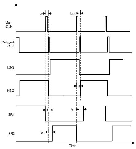
Figure 7-7. PWM Signals at Maximum Duty Cycle Condition
