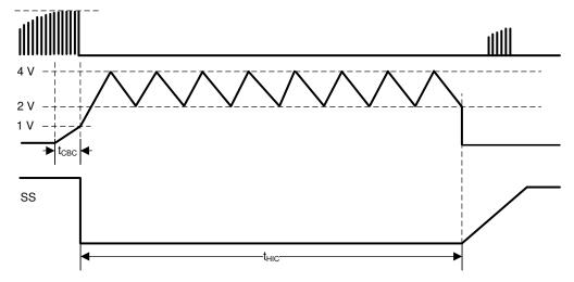
Figure 7-18. Hiccup Mode Activated By Continuous CBC Operation
