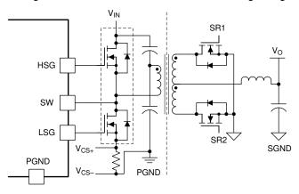
Figure 7-11. Half-Bridge Converter with Low-Side Current Sensing
