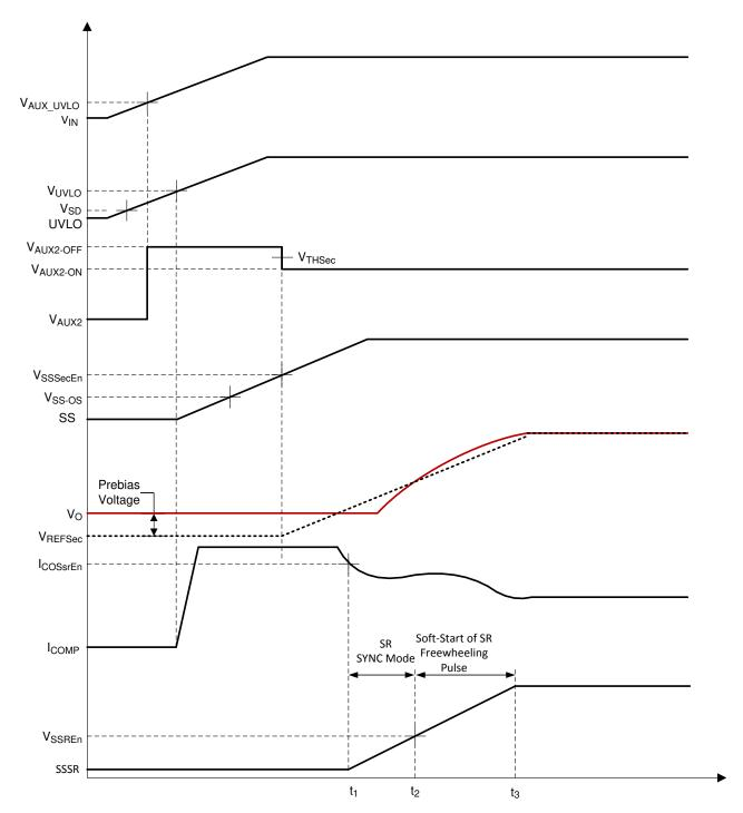
Figure 7-9. Pre-biased Start-Up Waveform
