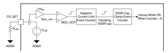
Figure 7-15. Reverse Current Protection Circuit
