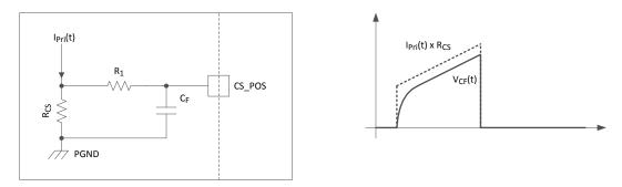
Figure 8-10. CS\_POS Filter Circuit Model and Waveform
