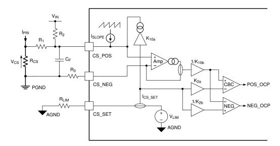
Figure 7-12. Block Diagram of the Current Limiting Function
