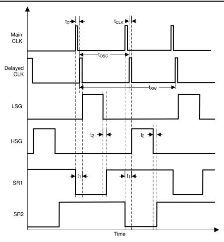
Figure 7-6. PWM Signal Timing Diagram
