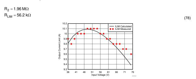
Figure 8-9. Main Converter Measured vs Predicted Output Current Limit
