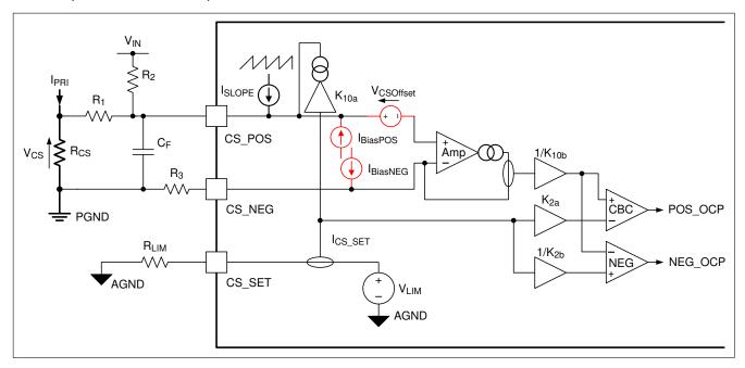
Figure 7-16. Diagram of Current Limiting Function with Error Terms Shown in Red
