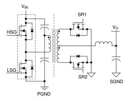
Figure 7-5. Half-bridge Topology with Center-Tap Rectification
