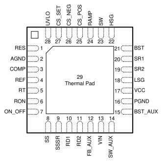
Figure 5-1. RJB Package, 28-Pin WQFN (Top View)
