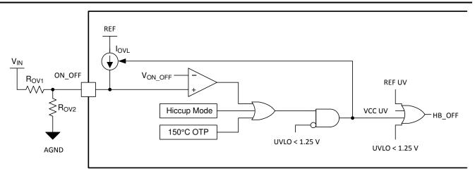
Figure 7-21. ON/OFF Pin Configured as OVP Pin
