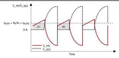
Figure 7-26. Auxiliary Transformer Current Waveform for CAUX1 Ripple Calculation
