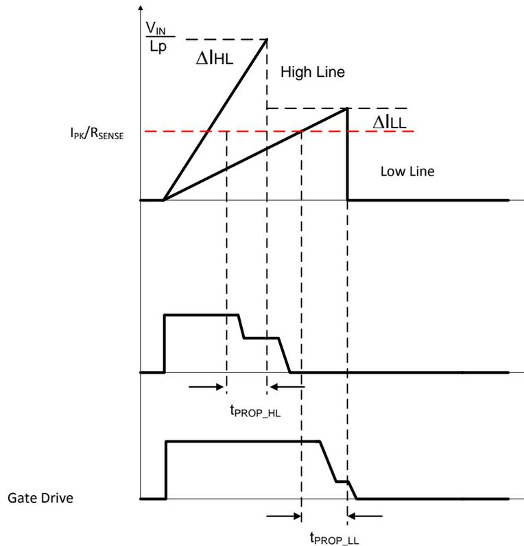
**Figure 15. Line-Current Feedforward**
