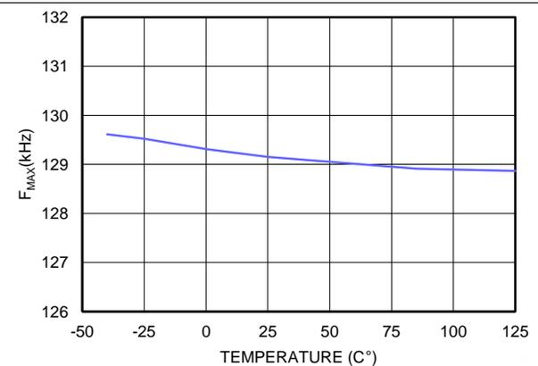
Figure 7. F<sub>MAX</sub> vs. Temperature
