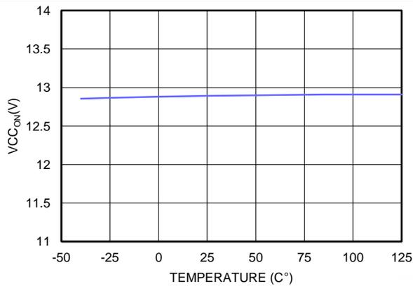
Figure 2. VCC<sub>ON</sub> vs. Temperature
