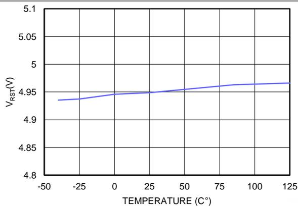
Figure 4. V<sub>RST</sub> vs. Temperature
