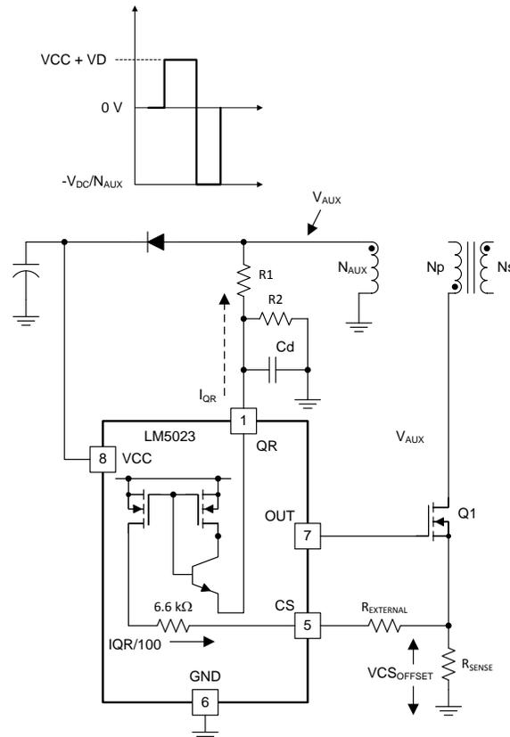
Figure 16. Current Feedforward
