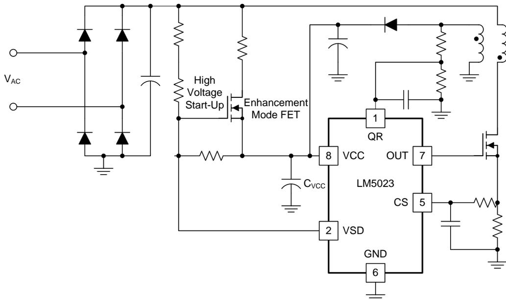
**Figure 10. Start-Up With an Enhancement Mode FET**
