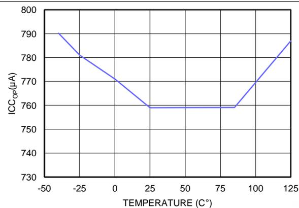
Figure 6. ICC<sub>OP</sub> vs. Temperature
