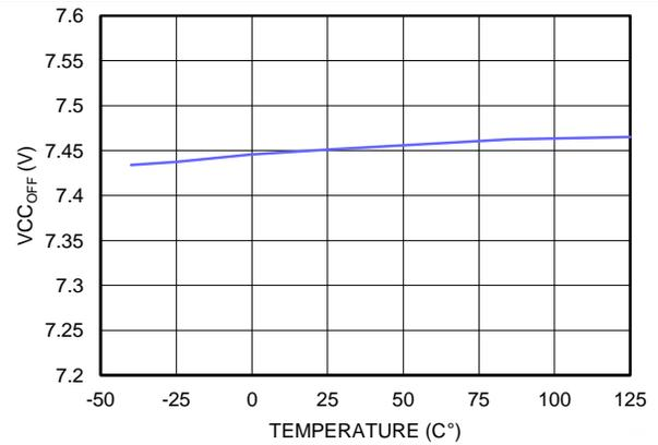
Figure 3. VCC<sub>OFF</sub> vs. Temperature
