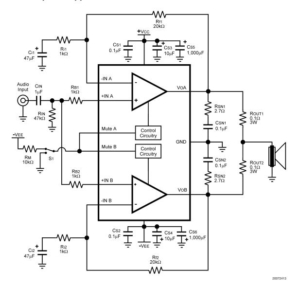
FIGURE 3. Parallel Amplifier Application Circuit
