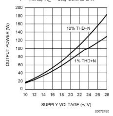
Output Power vs Supply Voltage, Parallel Mode (Note 17)  $f=1 kHz, \ R_L=4 \Omega, \ 80 kHz \ BW$
