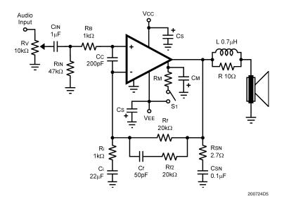
FIGURE 5. Special Audio Amplifier Application Circuit
