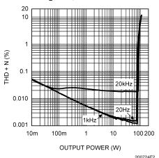
THD+N vs Output Power  $\pm$  29V, Parallel Mode (Note 17) R<sub>L</sub> =  $4\Omega$ , 80kHz BW
