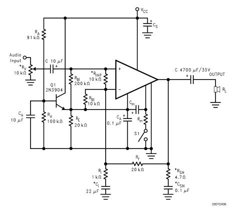
FIGURE 4. Single Supply Amplifier Application Circuit
