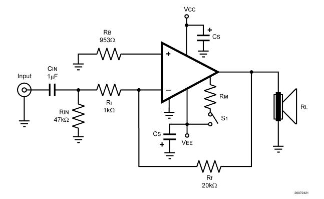
FIGURE 6. Inverting Amplifier Application Circuit
