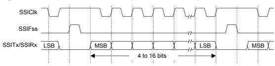
Figure 11-8. Freescale SPI Frame Format (Continuous Transfer) with SPO=1 and SPH=0
