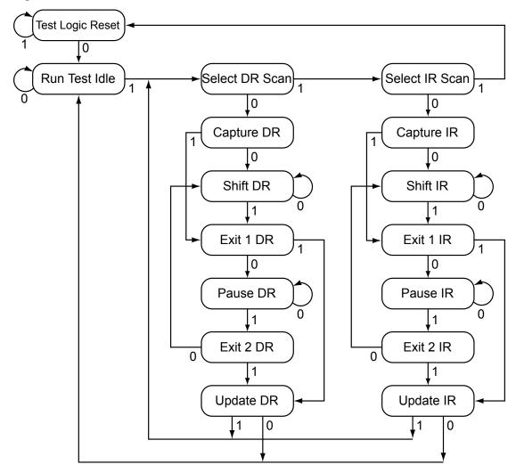
Figure 4-2. Test Access Port State Machine
