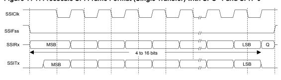
Figure 11-7. Freescale SPI Frame Format (Single Transfer) with SPO=1 and SPH=0
