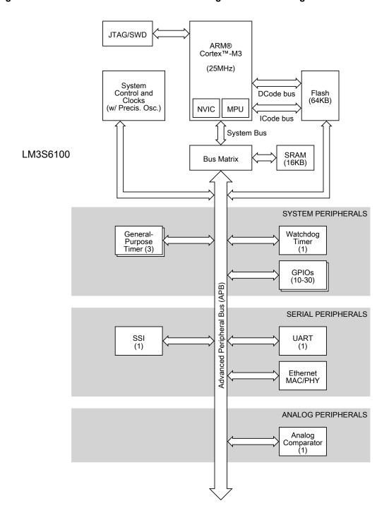
Figure 1-1. Stellaris LM3S6100 Microcontroller High-Level Block Diagram
