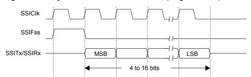
Figure 11-2. TI Synchronous Serial Frame Format (Single Transfer)
