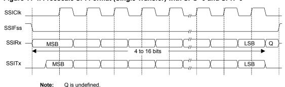
Figure 11-4. Freescale SPI Format (Single Transfer) with SPO=0 and SPH=0
