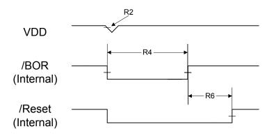
Figure 17-8. Software Reset Timing
