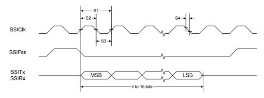
Figure 17-11. SSI Timing for MICROWIRE Frame Format (FRF=10), Single Transfer
