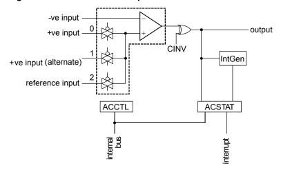
A comparator is configured through two status/control registers (ACCTL and ACSTAT). The internal reference is configured through one control register (ACREFCTL). Interrupt status and control is configured through three registers (ACMIS, ACRIS, and ACINTEN).
