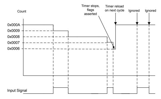
Figure 8-2. 16-Bit Input Edge Count Mode Example
