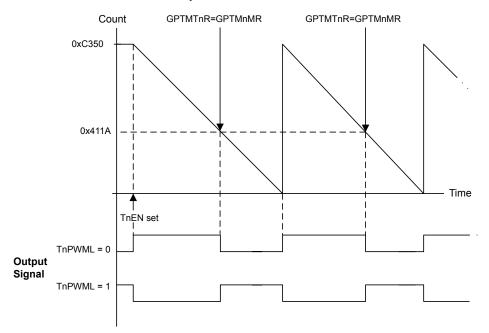
Figure 8-4. 16-Bit PWM Mode Example
