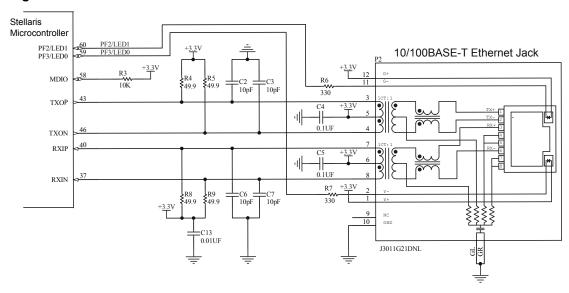
Figure 12-4. Interface to an Ethernet Jack
