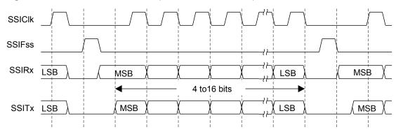
Figure 11-5. Freescale SPI Format (Continuous Transfer) with SPO=0 and SPH=0
