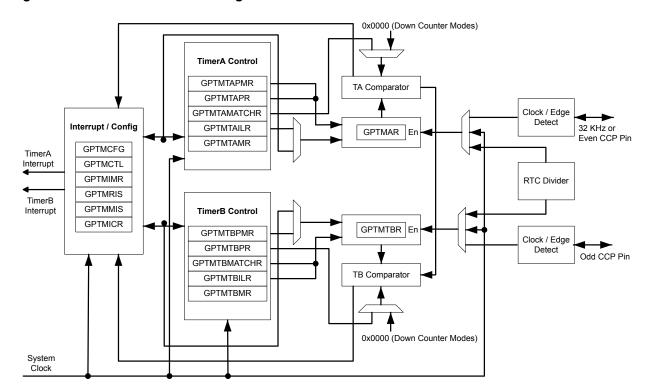
Figure 8-1. GPTM Module Block Diagram
