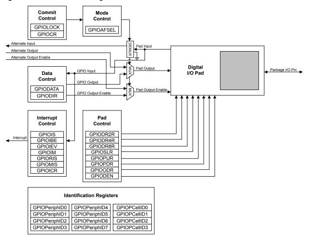
Figure 7-1. GPIO Port Block Diagram
