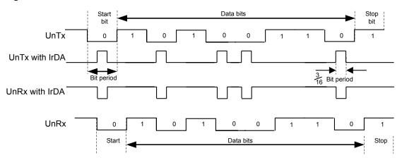
Figure 10-3. IrDA Data Modulation
