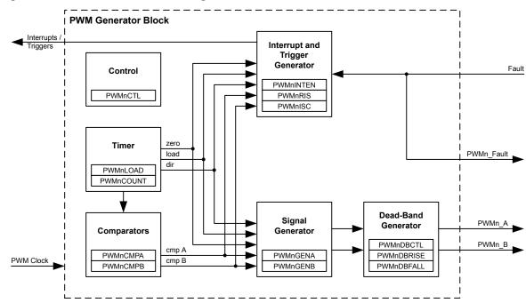
Figure 19-2. PWM Module Block Diagram
