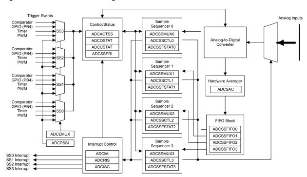
Figure 12-1. ADC Module Block Diagram
