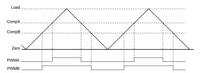
Figure 19-5. PWM Generation Example In Count-Up/Down Mode
