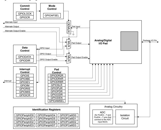
Figure 9-2. Analog/Digital I/O Pads
