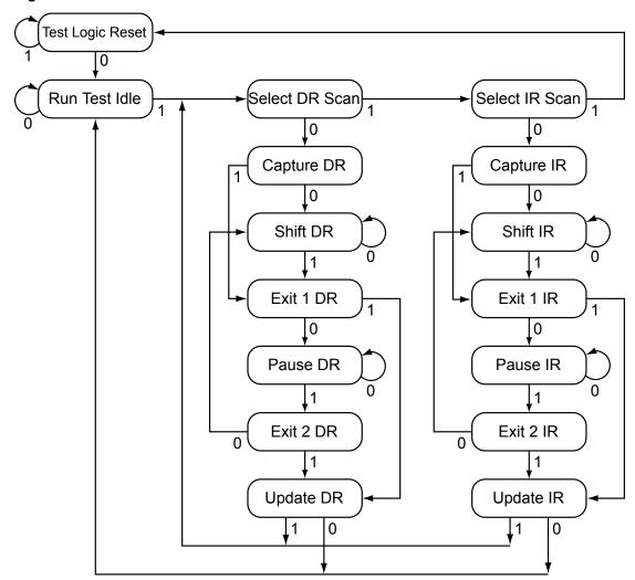
Figure 4-2. Test Access Port State Machine
