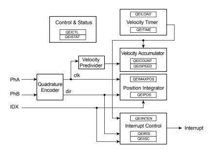
Figure 20-1. QEI Block Diagram
