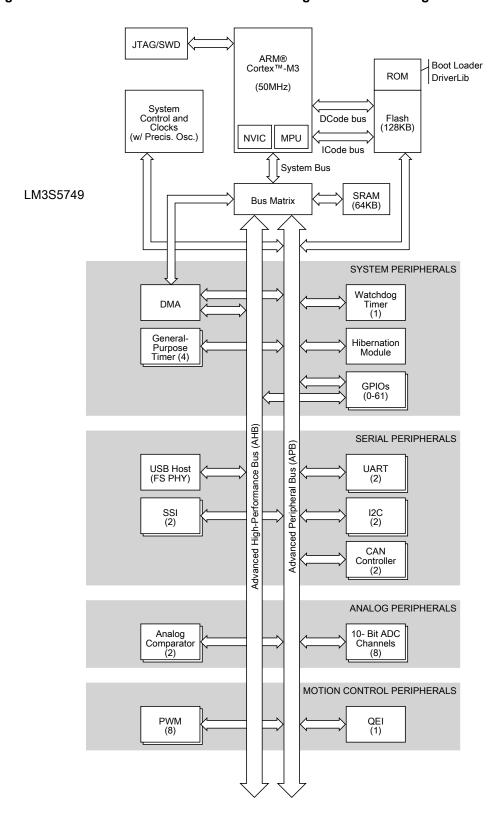
Figure 1-1. Stellaris LM3S5749 Microcontroller High-Level Block Diagram
