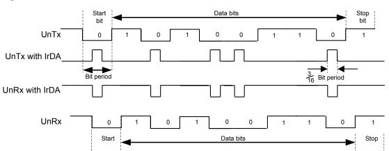
Figure 13-3. IrDA Data Modulation
