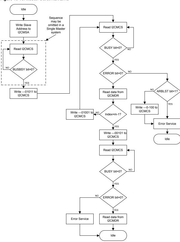
Figure 15-10. Master Burst RECEIVE
