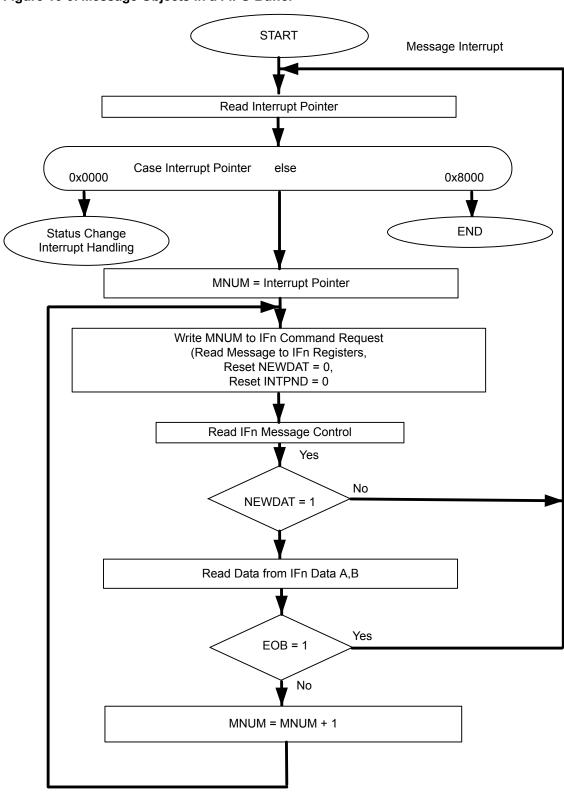
Figure 16-3. Message Objects in a FIFO Buffer
