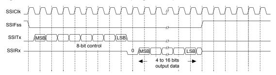
Figure 14-10. MICROWIRE Frame Format (Single Frame)
