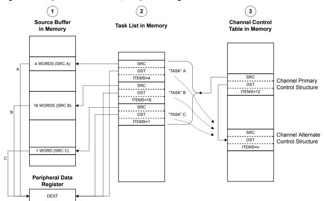
Figure 8-5. Peripheral Scatter-Gather, Setup and Configuration
