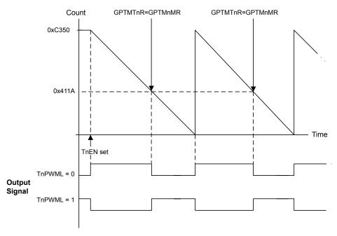
Figure 10-4. 16-Bit PWM Mode Example
