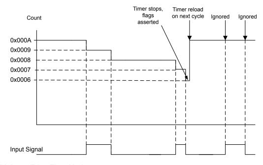
Figure 10-2. 16-Bit Input Edge Count Mode Example
