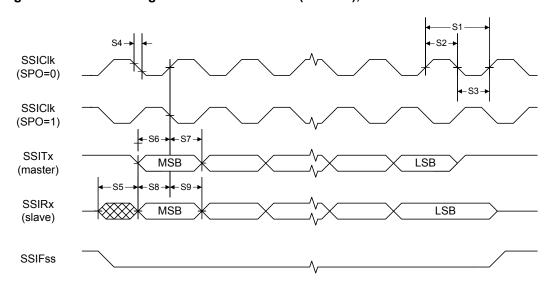
Figure 24-13. SSI Timing for SPI Frame Format (FRF=00), with SPH=1
