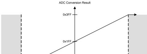
Figure 12-2. Differential Sampling Range,  $V_{IN\_ODD}$  = 1.5 V
