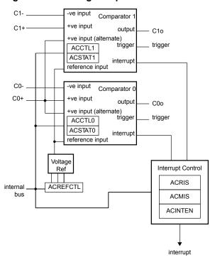
Figure 18-1. Analog Comparator Module Block Diagram
