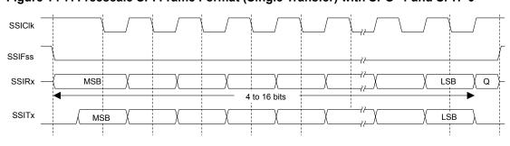
Figure 14-7. Freescale SPI Frame Format (Single Transfer) with SPO=1 and SPH=0
