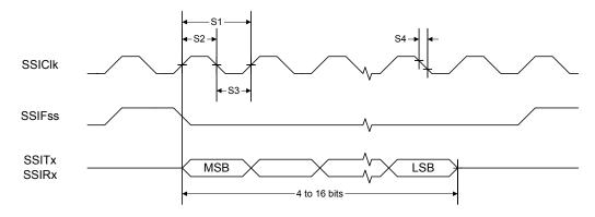
Figure 24-12. SSI Timing for MICROWIRE Frame Format (FRF=10), Single Transfer
