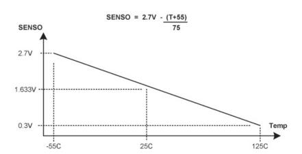
Figure 12-5. Internal Temperature Sensor Characteristic
