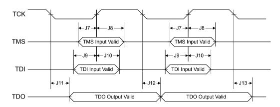
Figure 24-3. JTAG Test Access Port (TAP) Timing
