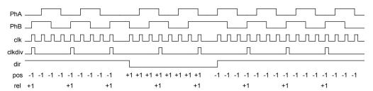
Figure 20-2. Quadrature Encoder and Velocity Predivider Operation
