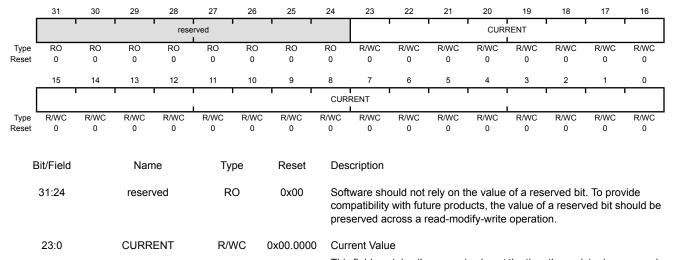
This field contains the current value at the time the register is accessed. No read-modify-write protection is provided, so change with care.
