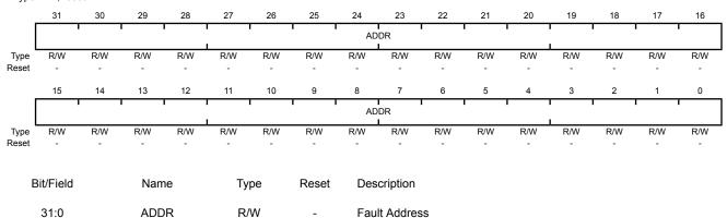
When the  ${\tt MMARV}$  bit of **MFAULTSTAT** is set, this field holds the address of the location that generated the memory management fault.
