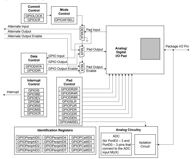
Figure 8-2. Analog/Digital I/O Pads
