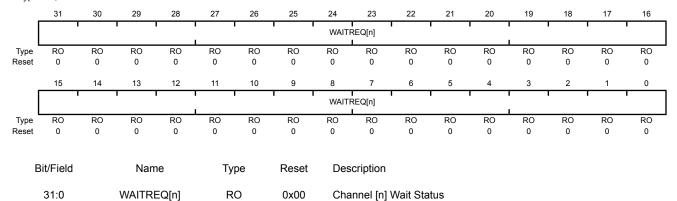
Channel wait on request status. For each channel 0 through 31, a 1 in the corresponding bit field indicates that the channel is waiting on a request.
