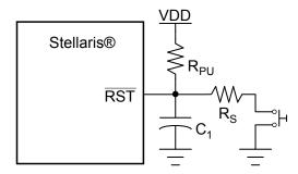
Typical  $R_{PU} = 10 \text{ k}\Omega$
