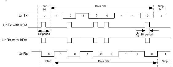
Figure 12-3. IrDA Data Modulation
