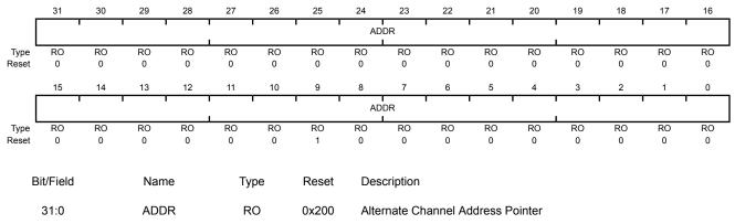
Provides the base address of the alternate channel control structures.
