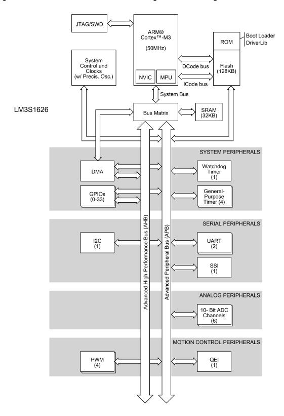
Figure 1-1. Stellaris LM3S1626 Microcontroller High-Level Block Diagram
