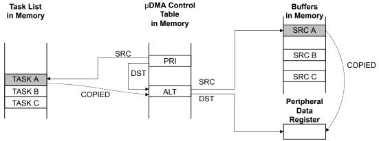
Using the channel's primary control structure, the  $\mu DMA$  controller copies task A configuration to the channel's alternate control structure.
