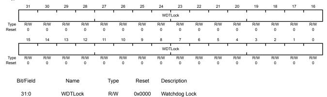
A write of the value 0x1ACC.E551 unlocks the watchdog registers for write access. A write of any other value reapplies the lock, preventing any register updates.
