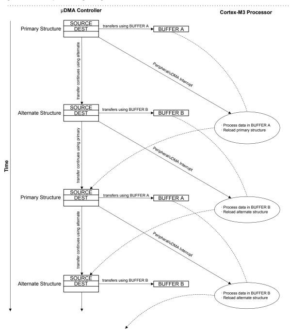
Figure 7-2. Example of Ping-Pong DMA Transaction
