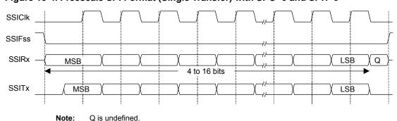
Figure 13-4. Freescale SPI Format (Single Transfer) with SPO=0 and SPH=0
