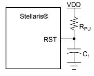
$R_{PU} = 1 k\Omega$  to 100  $k\Omega$
