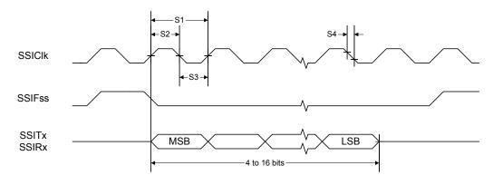
Figure 20-11. SSI Timing for MICROWIRE Frame Format (FRF=10), Single Transfer
