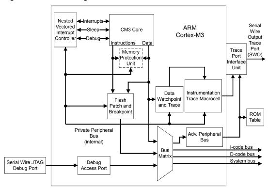
Figure 2-1. CPU Block Diagram
