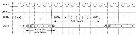
Figure 13-11. MICROWIRE Frame Format (Continuous Transfer)
