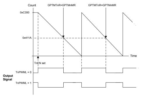
Figure 9-4. 16-Bit PWM Mode Example
