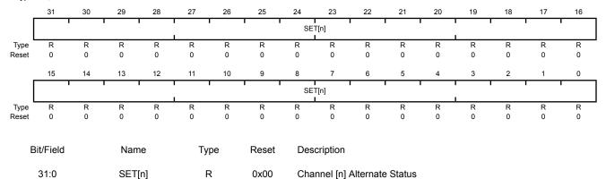
Channel [n] Alternate Status Returns the channel control data structure status.
