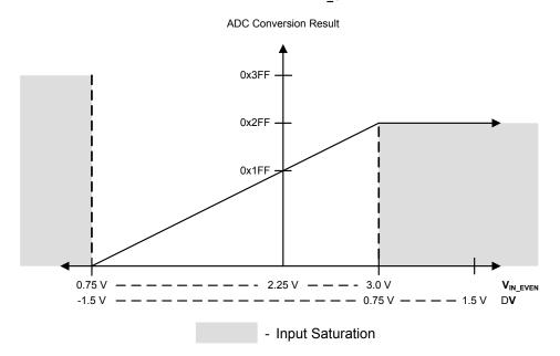
Figure 11-4. Differential Sampling Range,  $V_{IN\ ODD}$  = 2.25 V
