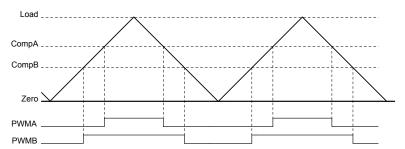
Figure 15-5. PWM Generation Example In Count-Up/Down Mode
