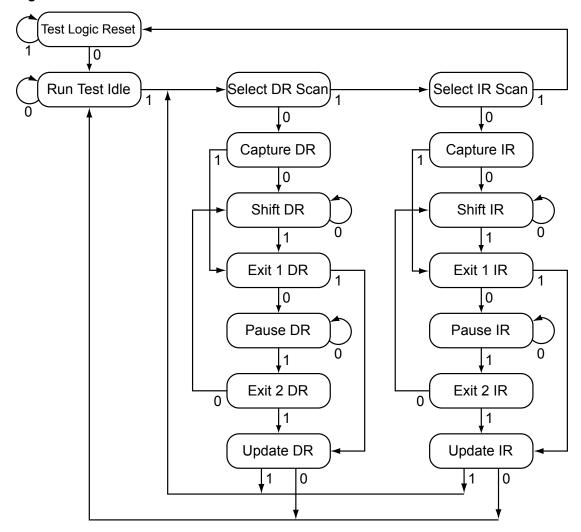
Figure 4-2. Test Access Port State Machine
