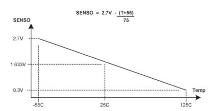
Figure 11-5. Internal Temperature Sensor Characteristic
