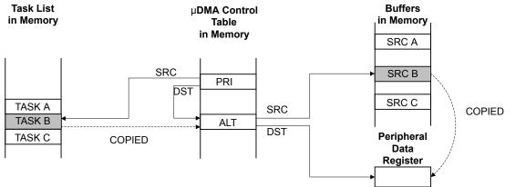
Using the channel's primary control structure, the  $\mu DMA$  controller copies task B configuration to the channel's alternate control structure.
