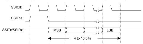
Figure 13-2. TI Synchronous Serial Frame Format (Single Transfer)
