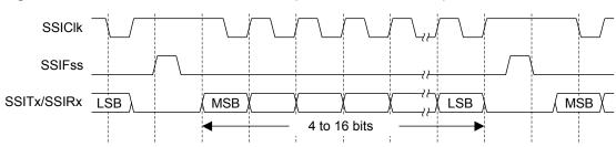
Figure 13-8. Freescale SPI Frame Format (Continuous Transfer) with SPO=1 and SPH=0
