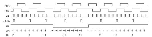
Figure 16-2. Quadrature Encoder and Velocity Predivider Operation
