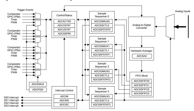
Figure 11-1. ADC Module Block Diagram
