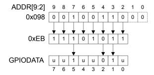
During a read, if the address bit associated with the data bit is set to 1, the value is read. If the address bit associated with the data bit is set to 0, it is read as a zero, regardless of its actual value. For example, reading address GPIODATA + 0x0C4 yields as shown in Figure 8-4 on page 328.
