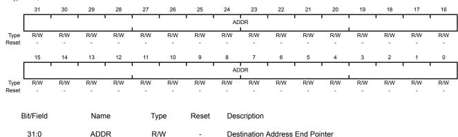
Points to the last address of the DMA transfer destination (inclusive). If the destination address is not incrementing, then this points at the destination location itself (such as a peripheral data register).
