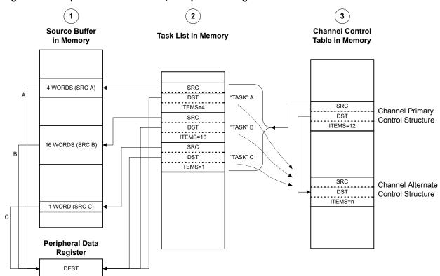
Figure 7-5. Peripheral Scatter-Gather, Setup and Configuration
