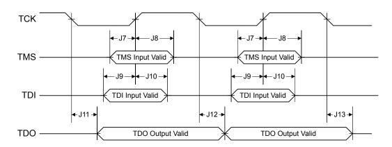
Figure 20-3. JTAG Test Access Port (TAP) Timing
