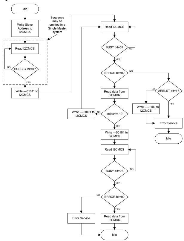
Figure 14-10. Master Burst RECEIVE
