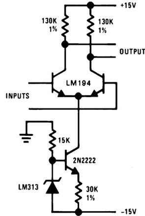
Figure 13. Amplifier Biasing for Constant Gain with Temperature
