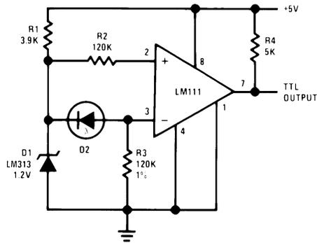
Figure 2. Level Detector for Photodiode
