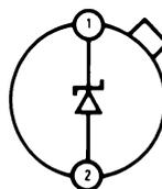
Note: Pin 2 connected to case.
