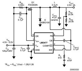
Typical High Efficiency Step-Down (Buck) Converter
