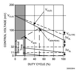
FIGURE 8. Current Limit and Hysteretic Threshold vs Duty Cycle with  $\rm R_{SL}$
