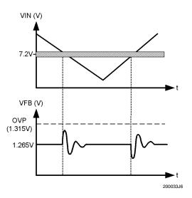
FIGURE 3. The Feedback Voltage Experiences an Oscillation if the Input Voltage Crosses the 7.2V Internal Bias Threshold
