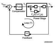
FIGURE 12. Control Block Diagram of a Current Mode Controlled Buck Converter
