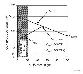
FIGURE 7. Current Limit and Hysteretic Threshold vs
