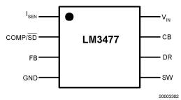
8 Lead Mini SO8 Package (MSOP-8 Package)
