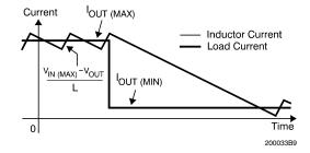
FIGURE 9. A Loading Transient
