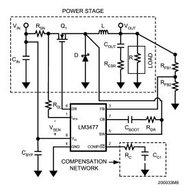
FIGURE 6. LM3477 Buck Converter Reference Schematic
