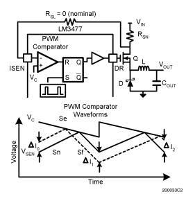
FIGURE 4. The Current Sensing Loop and Corresponding Waveforms
