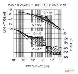
FIGURE 16. The Quality Factor Q of the Two Complex Poles is used to qualify how much resonant peaking is observed in the Power Stage Bode Plot
