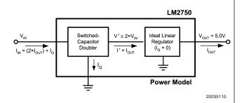
FIGURE 2. LM2750 Model for Power Efficiency and Power Dissipation Calculations
