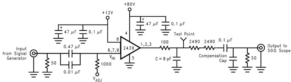
**Note:** 8 pF load includes parasitic capacitance.
