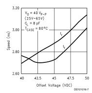
FIGURE 7. Speed vs Offset
