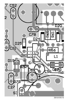
FIGURE 13. PCB CRT Driver, Blue Channel Output
