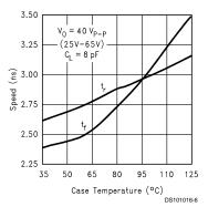
FIGURE 4. Speed vs Temp.
