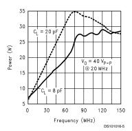
FIGURE 6. Power Dissipation vs Frequency
