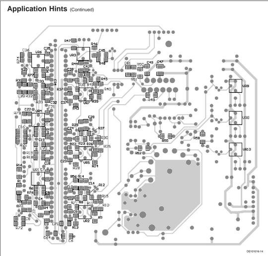
FIGURE 12. PCB Bottom Layer
