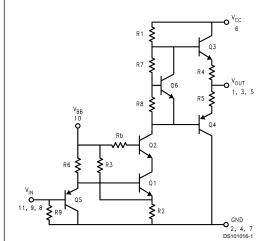
FIGURE 1. Simplified Schematic Diagram (One Channel)
