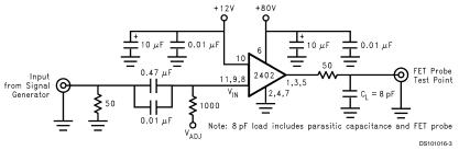
FIGURE 2. Test Circuit (One Channel)
