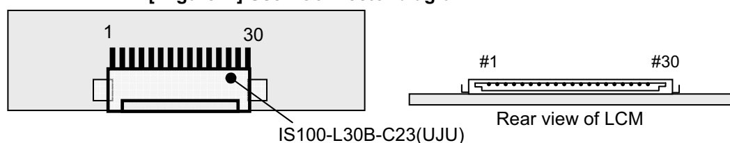
[ Figure 4 ] User Connector diagram
