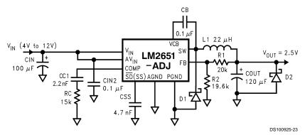
Schematic for the Typical Board Layout
