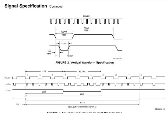
FIGURE 3. Equalization/Serration Interval Programming
