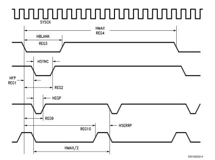
FIGURE 1. Horizontal Waveform Specification
