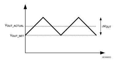
It can be seen that the average output voltage (VOUT\_ACTUAL) is higher than the output voltage (VOUT\_SET) that was calculated by the earlier equation by exactly half the output voltage ripple. The output voltage that is targeted for regulation may then be appended according to the voltage ripple. This can be seen below:
