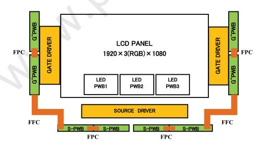
Layout of LED-PWB, S-PWB & G-PWB (Front View)
