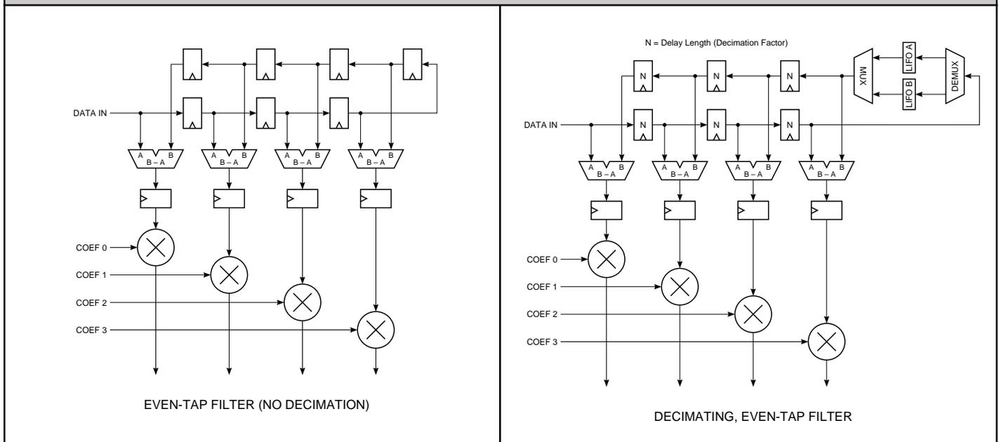
Figure 5 shows the two possible configurations when the device is programmed as a decimating, even-symmetric coefficient filter. The delay length of the decimation registers will be equal to the decimation factor that the device is programmed for. Since only four coefficients (effectively eight) can be sent to the filter multipli-
