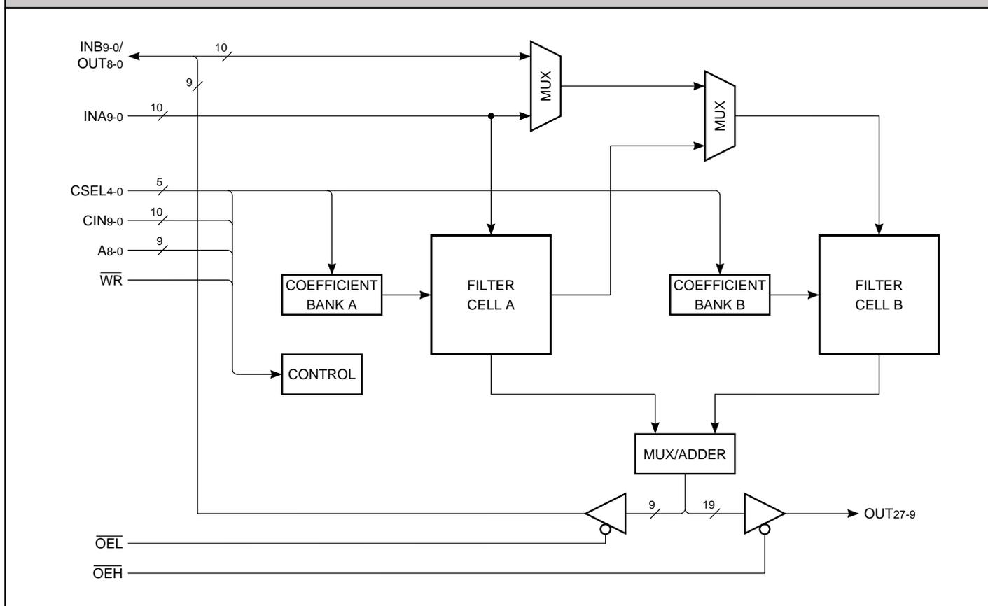
**FIGURE 1. LF43168 FUNCTIONAL BLOCK DIAGRAM**
