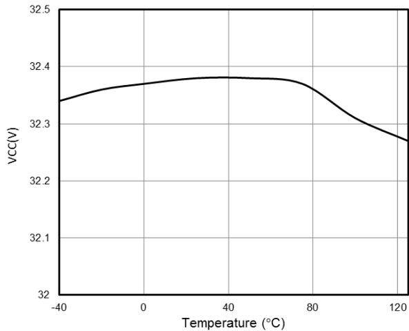
Fig. 4 VCC OVP vs. Temperature
