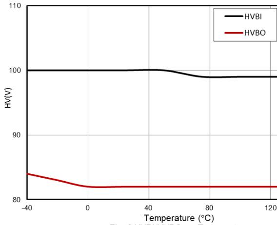
Fig. 2 HVBI/HVBO vs. Temperature
