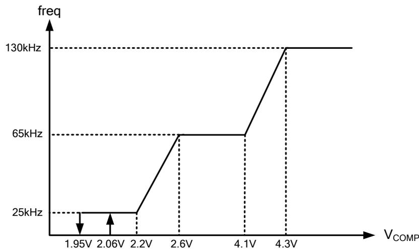
Fig. 1 V<sub>COMP</sub> vs. PWM Frequency
