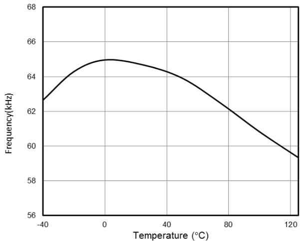
Fig. 5 Frequency Normal mode vs. Temperature
