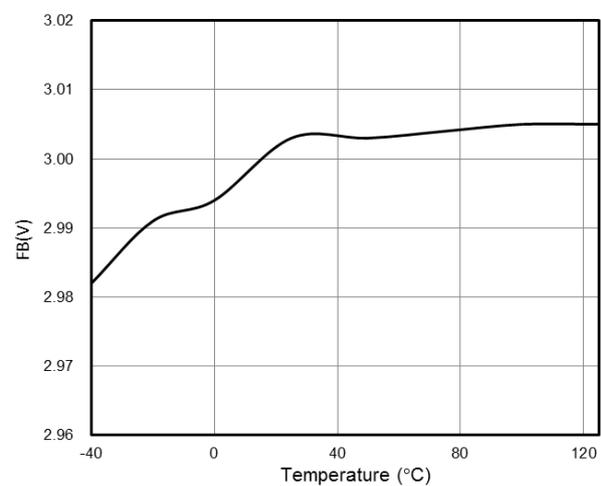
Fig. 7 FB OVP vs. Temperature
